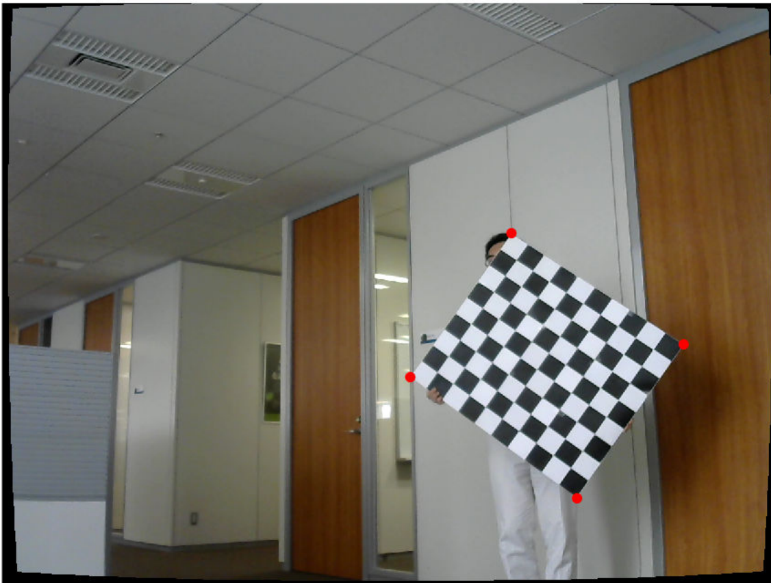
Detected Checkerboard Corners
